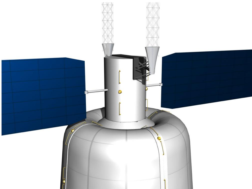
**Figure 30. Inflatable AG\_HAB Concept, subsystems module with tether reel.**
